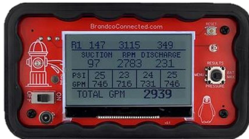
*Pump & Stream Sender recorded data shown at top*
