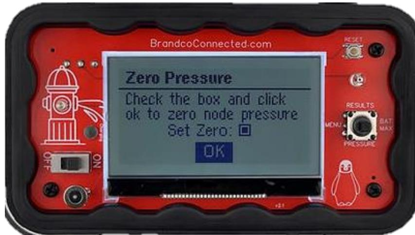
Check the Set Zero box and scroll down to OK. When you select OK the display will send a command to the Sender(s) to set zero pressure. The Sender's status light will flash yellow 3 times indicating it received the command and re-zero. It will return to normal operation after it is complete.
