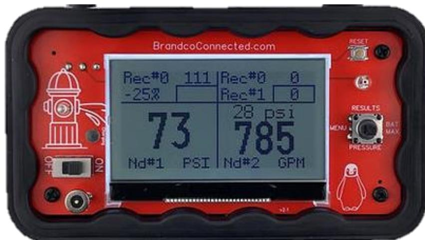
*Real time view of 2 Pressure Senders - the 2nd with flow calc enabled*
